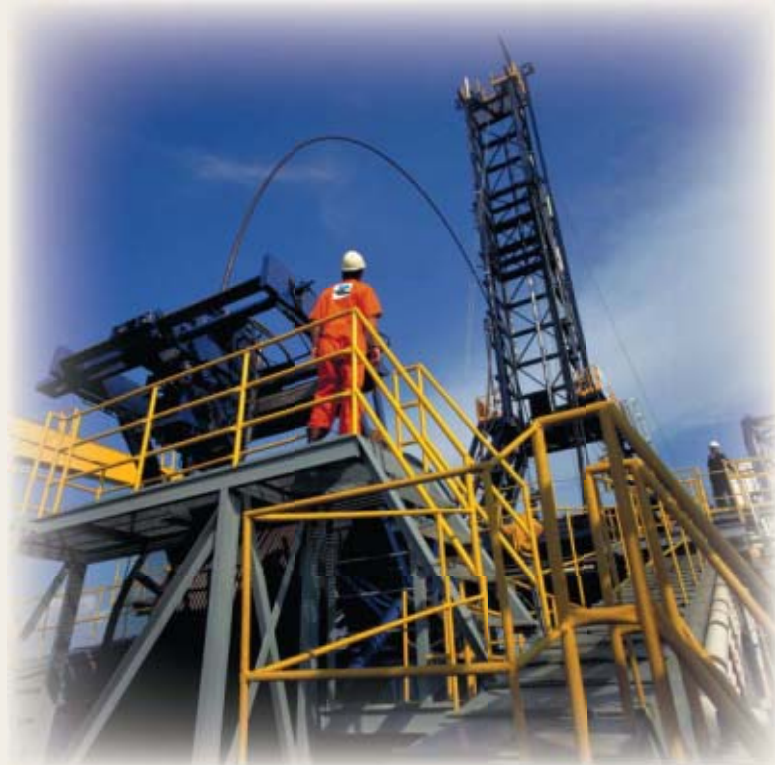
A hybrid coiled tubing drilling and well intervention unit developed by Baker Hughes is shown at work. Photo courtesy of Baker Oil Tools.
